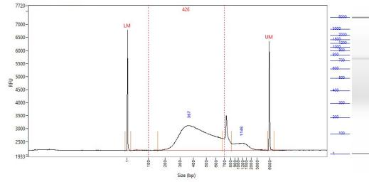
**Figure 6** An example of an over-tagmented library profile with a peak at 187 bp and an adapter peak at 42 bp
